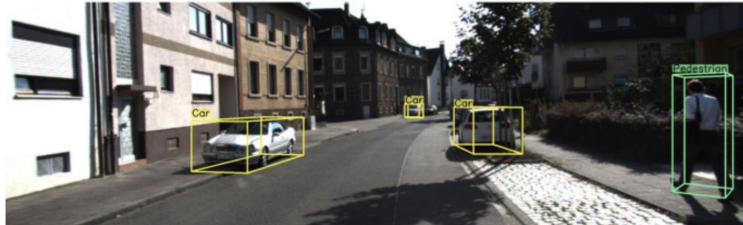
Monocular 3D Object Detection draws 3D bounding boxes on RGB images (source: M3D-RPN )
